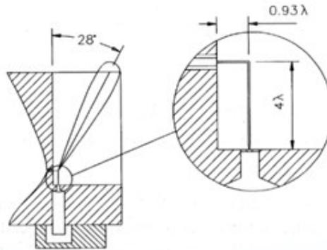
Figure 2. Corner Cube Mixer have 24° wide (at 10dB points) Gaussian beam at an angle of 28° to the vertical
