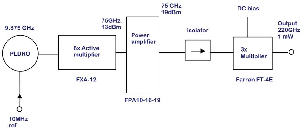
220GHz Low noise phase locked source
