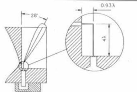
Figure 1. The corner cube detectors have a 24° wide (at 10dB points) Gaussian beam at an angle of 28° to the vertical.
